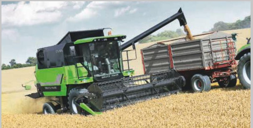
Unloading tube to discharge the grain while working in any position to tall trailer.
