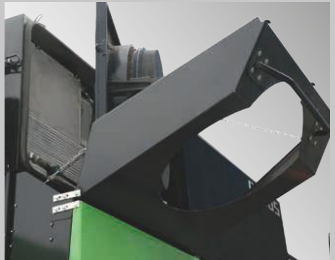
Big rotary screen to ensure maximum efficiency of the cooling system.
