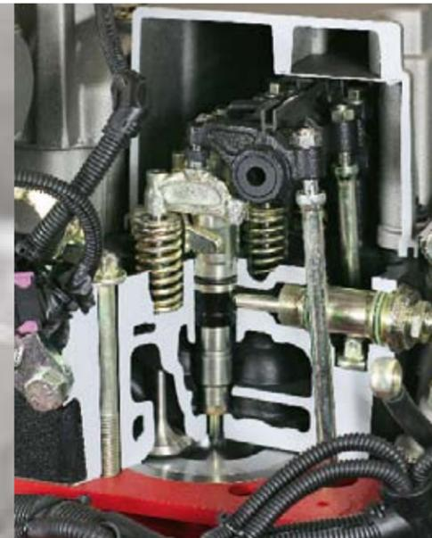
Four-valve, 6-hole injection nozzles optimize fuel consumption.
