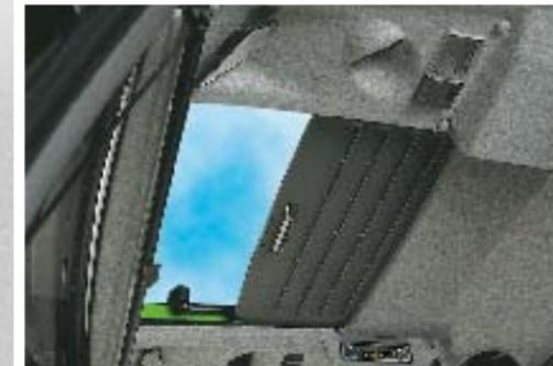
The roof hatch has a retractable screen for shade.
