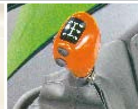
Six-speed main transmission and the four Powershift stages are operated on the gearshift lever.
