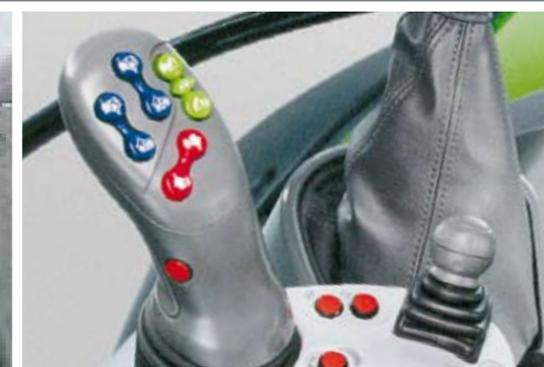
Use the PowerComS operating lever to shift to Powershift stages with just a touch.
